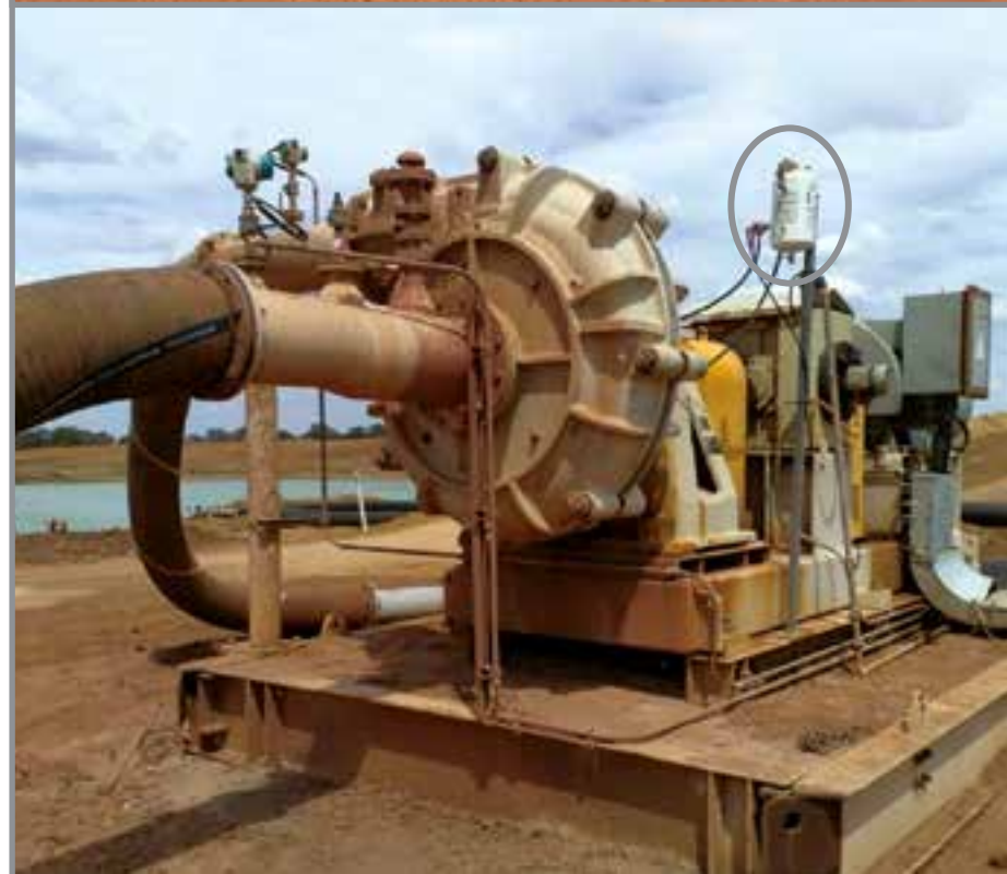
Below - Same Warman® slurry pump, AFTER installation of double mechanical seal and tank system (circled).
