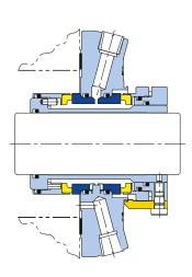
For seal chamber pressures ranging over 90barg (1305 PSIG) an engineered special is available with the below available options, application to be technically reviewed by the AESSEAL<sup>®</sup> technical department prior to ordering the seal. For additional material configurations please contact the technical department.
